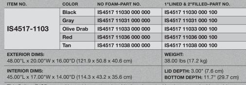
This Pelican™ ISP case with stacking pattern has black carbon steel hardware, two locking cable catches to lock the lid, PRV valve, a 3"x 5" cardholder, six comfort grip handles and mold-in edge casters for mobility. All six ISP case sizes cross-stack into each other no matter what the combination of case sizes, including cases with skid runners. Case is also configurable.
