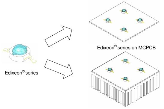
Edixeon® series on MCPCB and heat sink
